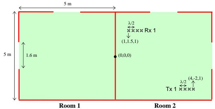
Figure 8: Geometry of the two rooms and the MIMO transmitter and receiver locations (top view).
